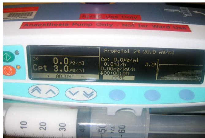
Fig. 4. Alaris PK syringe driver, loaded with generic propofol, with an indication of both  $C_p$  and  $C_e$  on the display: the solid line representing the predicted  $C_p$  and the dotted area representing  $C_e$ .
